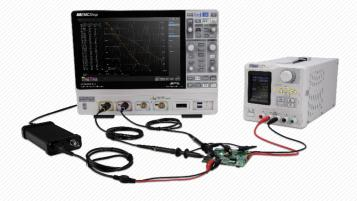
The oscilloscope can control the isolated USB AWG module or a stand-The EMC Shop The EMC Shop SDG generator, to scan the amplitude and phase-frequency response of the DUT, and display the data as a Bode Plot. This makes it possible to replace expensive network analyzers in some applications
