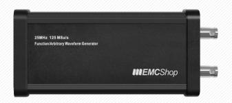
The oscilloscope can control isolated USB Function/Arbitrary waveform generator to output waveform with up to 25 MHz frequency and ±3 V amplitude. Six basic waveforms plus multiple types of arbitrary waveforms are built-in
