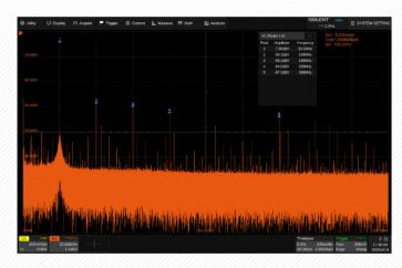
Hardware-accelerated FFT supports up to 8 Mpts operation. This provides high-frequency resolution with a fast refresh rate. The FFT function also supports a variety of window functions so that it can adapt to different spectrum measurement needs. Three modes (Normal, Average, and Max hold) can satisfy different requirements for observing the power spectrum. Auto peak detection and markers are supported.
